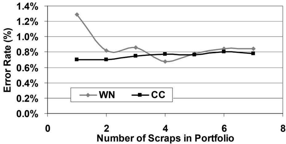
Figure 33. Comparing error rate for chance-constrained and window narrowing method for production of 100 kilotonne of 6061 alloy (COV=50%, 2 SD, WN=80%)
