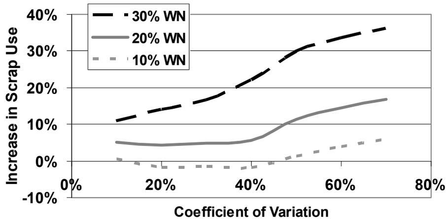
Figure 26. Improvement in scrap utilization of chance-constrained method over 30%, 20%, and 10% window narrowing methods (70%, 80%, and 90% windows) for a range of uncertainty conditions (SD=2) Base Case Comparison: COV=50%, 30% WN
