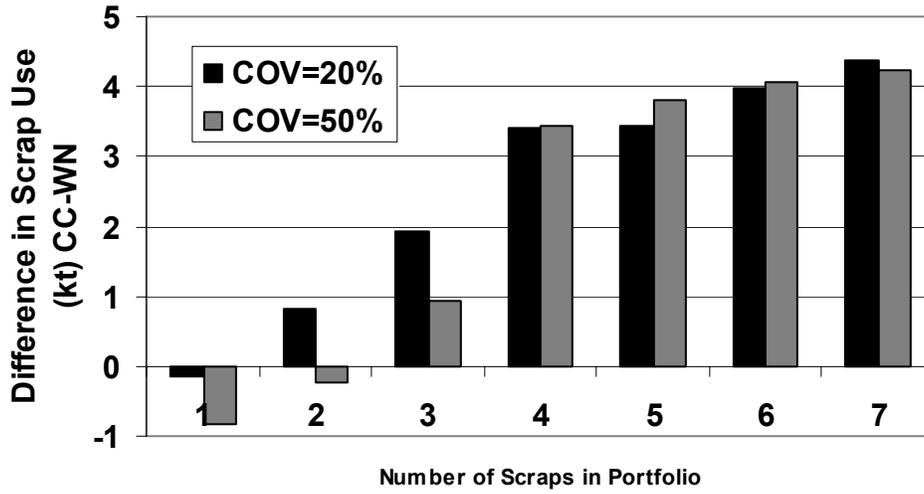
Figure 29. Scrap usage comparison between chance-constrained method and conventional window narrowing with increasing scrap portfolio diversification, taking away in order of least used (30% WN, COV=20%, 50%, SD=2)
