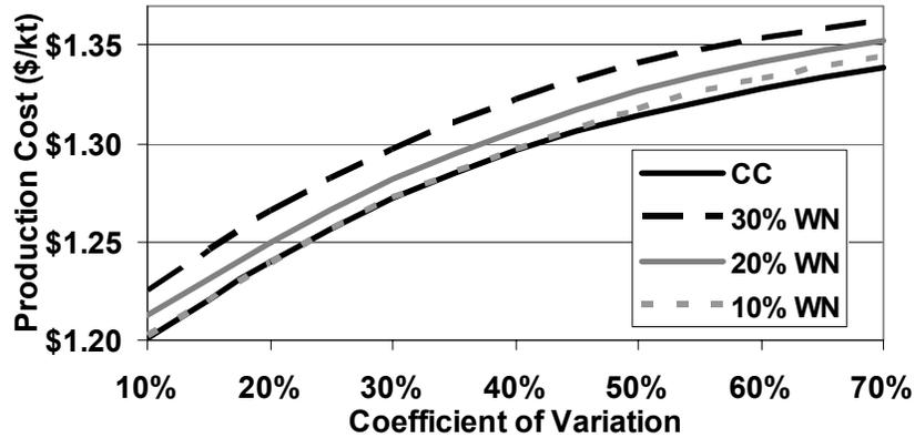
Figure 27. Improvement in production cost of chance-constrained method over 30%, 20%, and 10% window narrowing methods (70%, 80%, and 90% windows) for a range of uncertainty conditions (SD=2) Base Case Comparison: COV=50%, 30% WN
