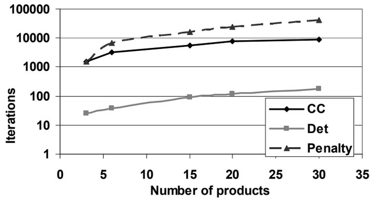
Figure 13. Number of iterations to global or local optimum convergence for the chance-constrained formulation (CC) and the penalty function formulation (Penalty) vs. the deterministic batch planning model (Det) with number of products
