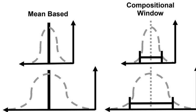
Figure 8. Schematic comparing the conventional methods for representing scrap composition as a mean or as a compositional window.
