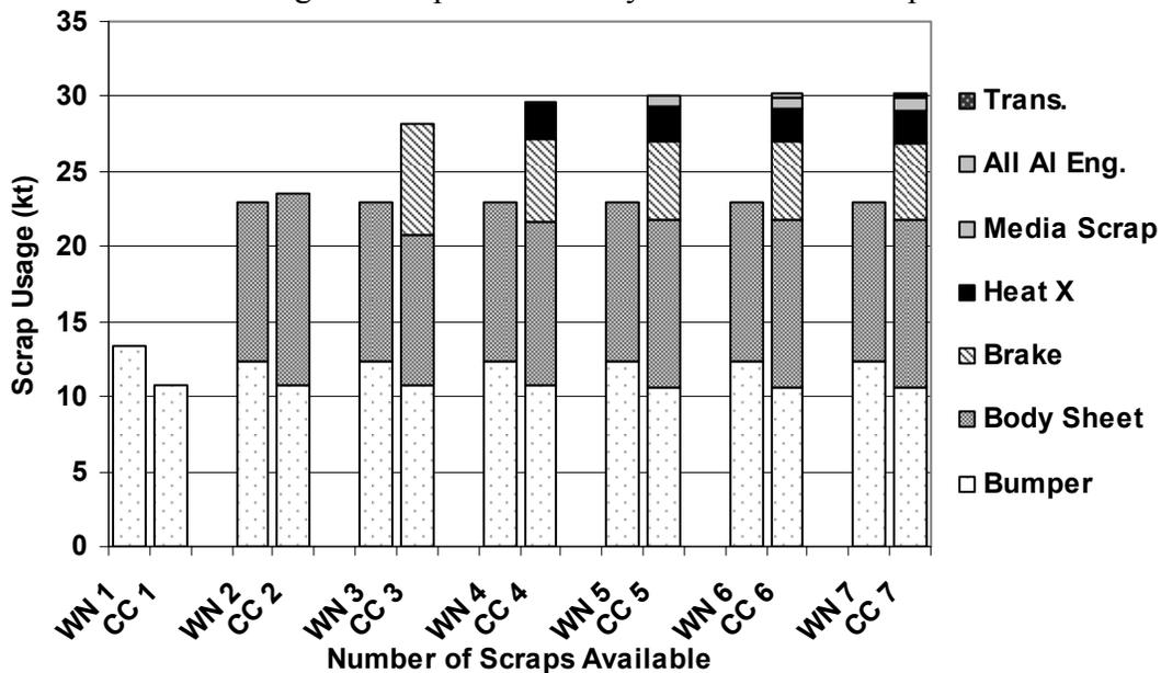
Figure 32. Comparison of detailed scrap consumption of chance-constrained (CC) and window narrowing (WN) methods with increasing scrap type availability. While the number of scraps available for consumption
