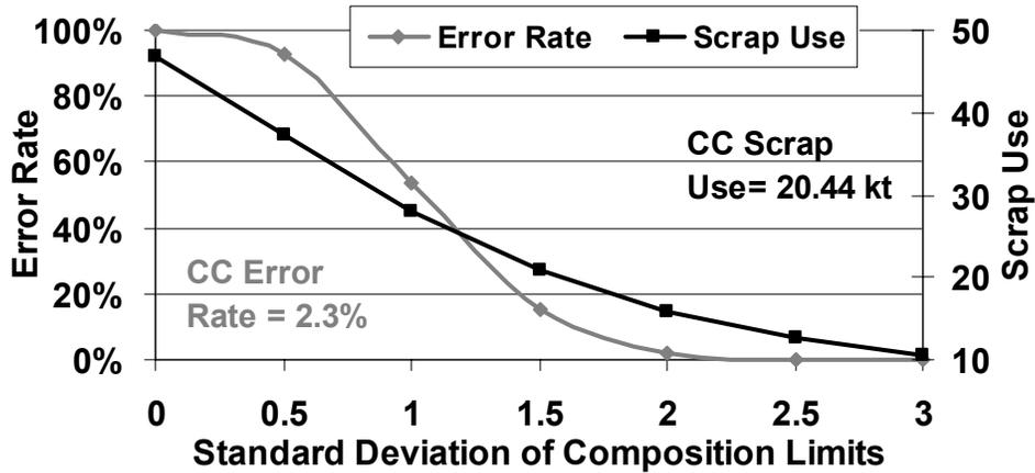
Figure 24. Scrap use and error rates for varying scrap compositional window representations for the window narrowing method (COV=50%, 30% WN). For a given variation in scrap composition, the finished good specification window size controls the error rate for this method. To maintain constant error rate, window size must be adjusted whenever scrap characteristics or availability change.
