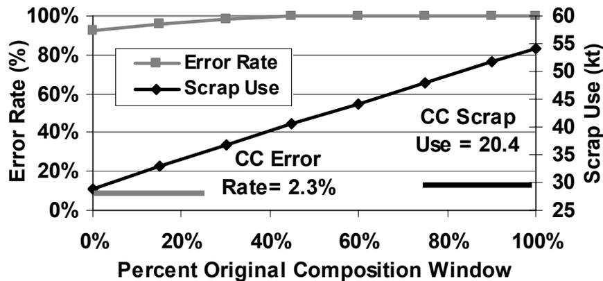
Figure 19. Error rates and scrap use for the mean based method at various degrees of window narrowing. Over all conditions, the error rate is much higher than the chance-constrained method when the COV=50%
