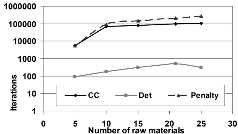
Figure 12. Number of iterations to global or local optimum convergence for the chance-constrained formulation (CC) and the penalty function formulation (Penalty) vs. the deterministic batch planning model (Det) with number of raw materials
