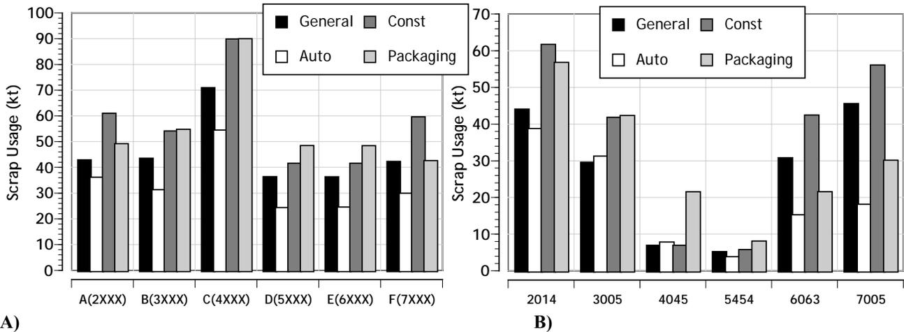
**Figure 38. Recycling friendly alloy set R (A) and market alloy (B) set M1 scrap use comparison for each different scrap “scenario”**
