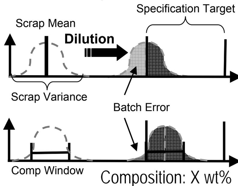
Figure 9. Schematic of scrap mixing illustrating the conventional method of representing scrap as a compositional window; when the window is set to be one standard deviation from the mean, a significant amount of batch errors will still occur
