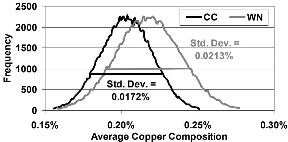
Figure 34. Comparison of stochastic Monte Carlo simulation of average copper composition for alloy 6061 produced according to production plans derived from either chance-constrained (CC) or window narrowing (WN) methods.
