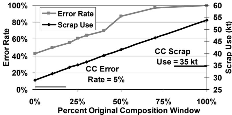
Figure 20. Error rates and scrap use for the mean based method at various degrees of window narrowing. At 75% window narrowing (25% original compositional window), the mean based method has equivalent scrap use to chance-constrained method but still a much higher error rate even with reduced variation (COV=20%)
