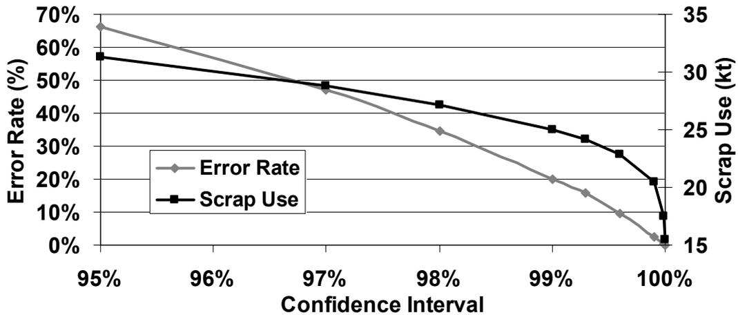
Figure 25. Scrap use and error rates for varying confidence intervals for the chance-constrained method. Error rate for the CC method is easily controlled through the alpha value specification and does not change significantly with scrap characteristics or availability. The base case alpha value of 99.90% gives a suitably low batch error rate.
