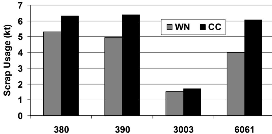
Figure 21. Comparison between base case results for chance-constrained and 30% window narrowing showing varying degrees of improved scrap consumption for the production of individual alloys (50% COV, 2 SD)
