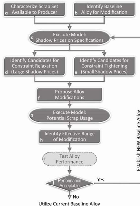
**Figure 43. Framework to identify alloy modification targets and possible recycling-friendly alloys**
