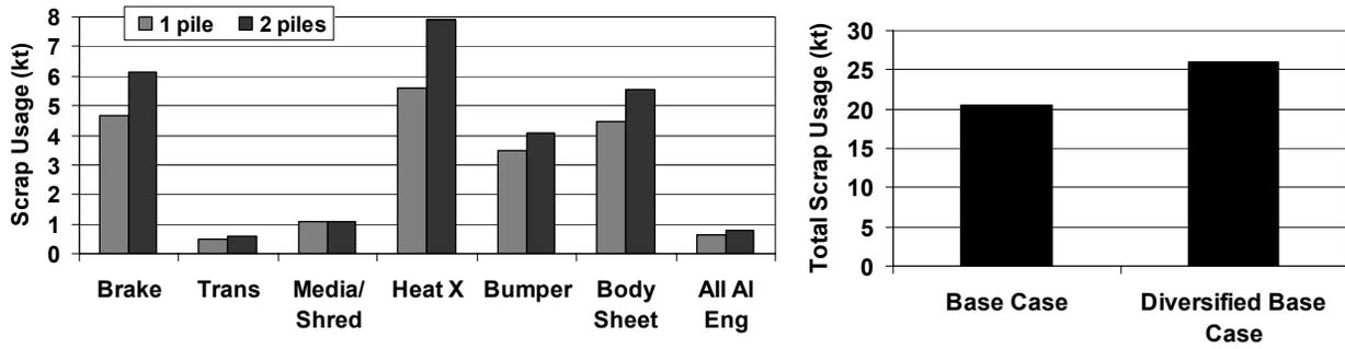
A) Comparison of individual scrap consumption when sampling from one or two piles of each scrap using the chance-constrained method B) Total effect of sampling diversification within the chance-constrained method (COV=50%)
