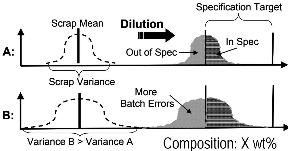
**Figure 7. Schematic of scrap mixing illustrating shortcomings of mean based conventional method. Typical mean-based optimizations cannot differentiate between scrap A (small variance) and scrap B (large variance).**
