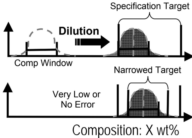
Figure 10. Scrap represented as compositional window combined with narrowed finished good specification targets: the window narrowing conventional method
