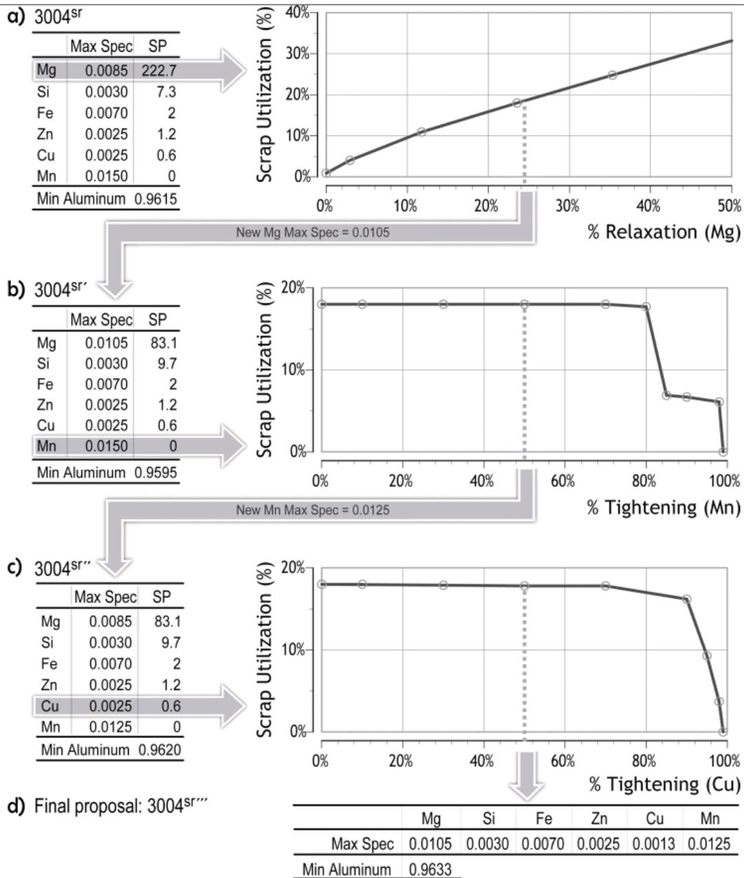
Figure 44. A) Improvement in scrap consumption of loosening Si constraints on alloy 3004, B) Effect on scrap consumption of now tightening other constraints in conjunction with loosening the Si constraint
