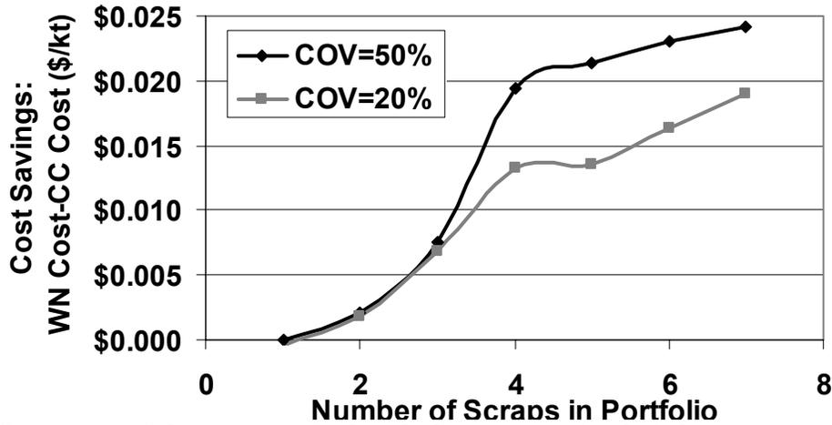
Figure 31. Cost savings of chance-constrained method over conventional window narrowing method with increasing scrap portfolio diversification (COV=20% or 50%, SD=2, WN=70%)
