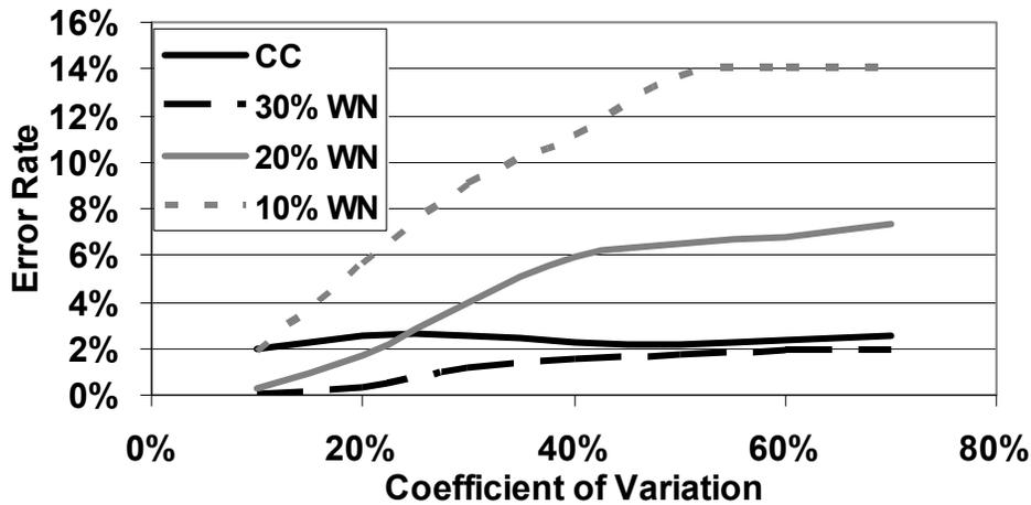
Figure 28. Fluctuating error rates with increasing scrap variability at various window sizes for all variations of window narrowing method. CC method maintains consistent error rates. Base Case Comparison: COV=50%, 30% WN, SD=2
