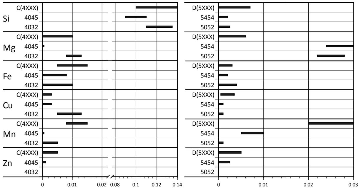
**Figure 41. Schematic representation of alloy compositional specification windows for the 4XXX and 5XXX series alloys of all three sets**
