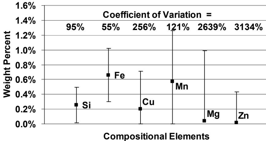
Figure 6. Compositional uncertainty (mean and standard deviation of various elements) in scrap aluminum siding sampled over the course of a year [4]
