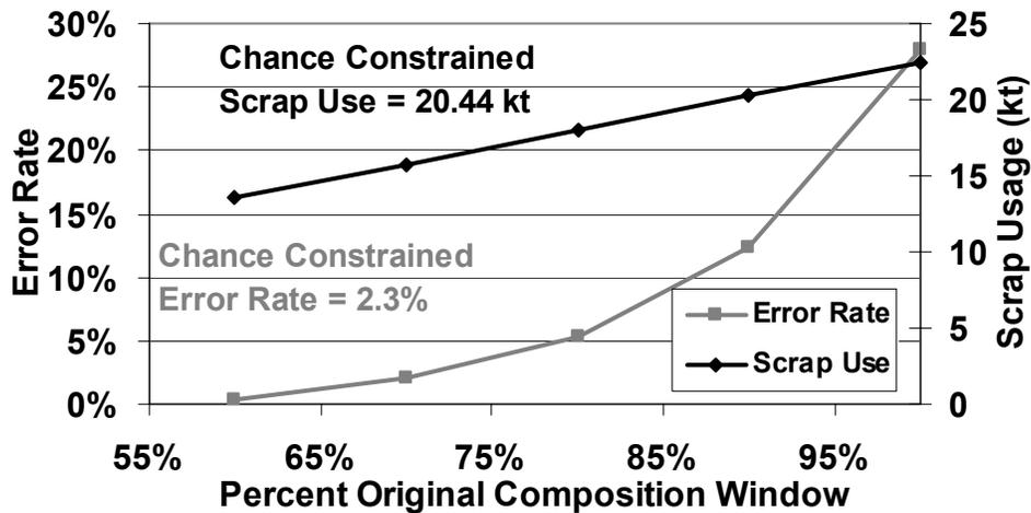
Figure 23. Scrap usage and error rate of the chance-constrained method compared to varying window sizes for the window narrowing method. A window narrowing size of 30% (70% original composition window) was chosen for the base case due to nearly equivalent error rate with the chance constrained method
