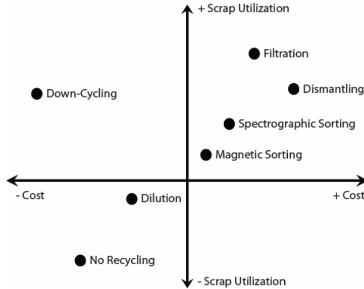
**Figure 48. The cost and scrap utilization trade-offs of various strategies for dealing with compositional accumulation**
