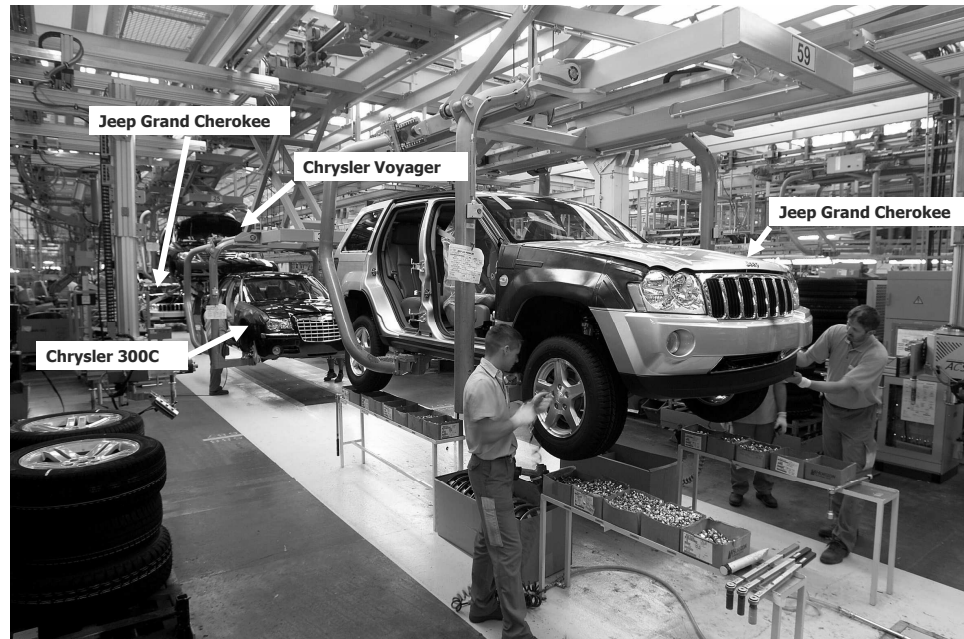
Figure 19: Three models on one assembly line (Daimler-Chrysler, courtesy: Magna)
