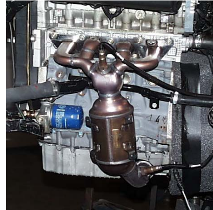
Figure 1. Example of a maniverter system
